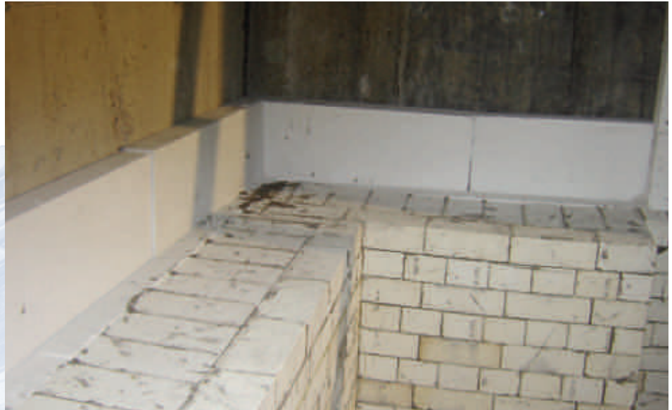
Chamber lining of an anode baking furnace with PROMASIL and PROMATON
