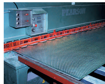
Production of DURASTEEL®-cut sections on the Promat cutting plant
